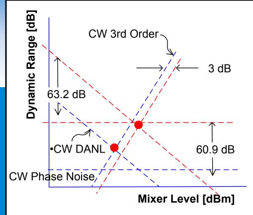
S/N Curve Offset: 10\* Log(1.23 MHz) +2.51 dB - .25 dB = 63.2 dB
