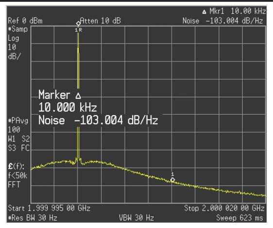
Phase noise measurement using noise marker function and delta (relative) calculation
