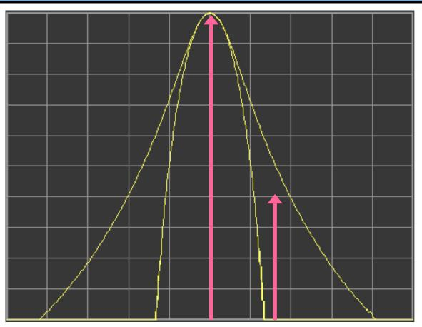
•Shape factor 4:1 vs. 12:1 enables viewing of close-in signals at wider (faster sweeping) RBW
